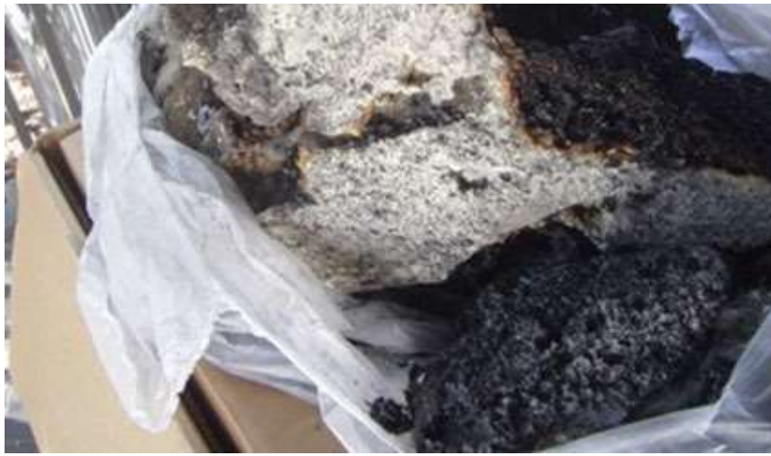
Four examples of fire damage from exothermic ignition from an excessive amount of foam applied in a single pass to fill and seal the soffit area. PHOTOS PROVIDED BY MASON KNOWLES
