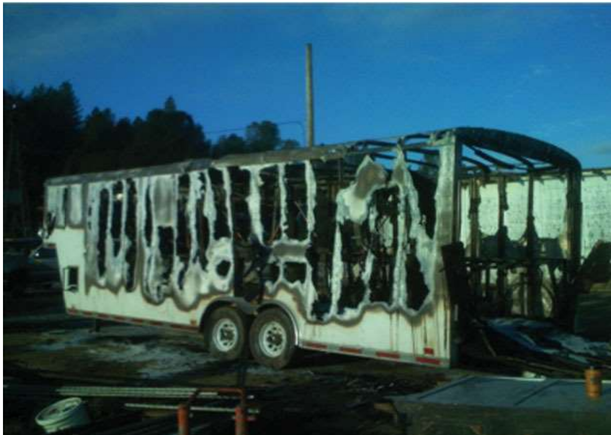
Rig destroyed by fire from overheated spray buns placed inside without
