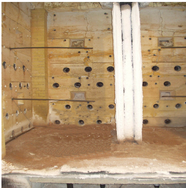
Figure 2—Fire Resistant Coating Char Development on a Structural Steel Column in ASTM E119 Fire Test
