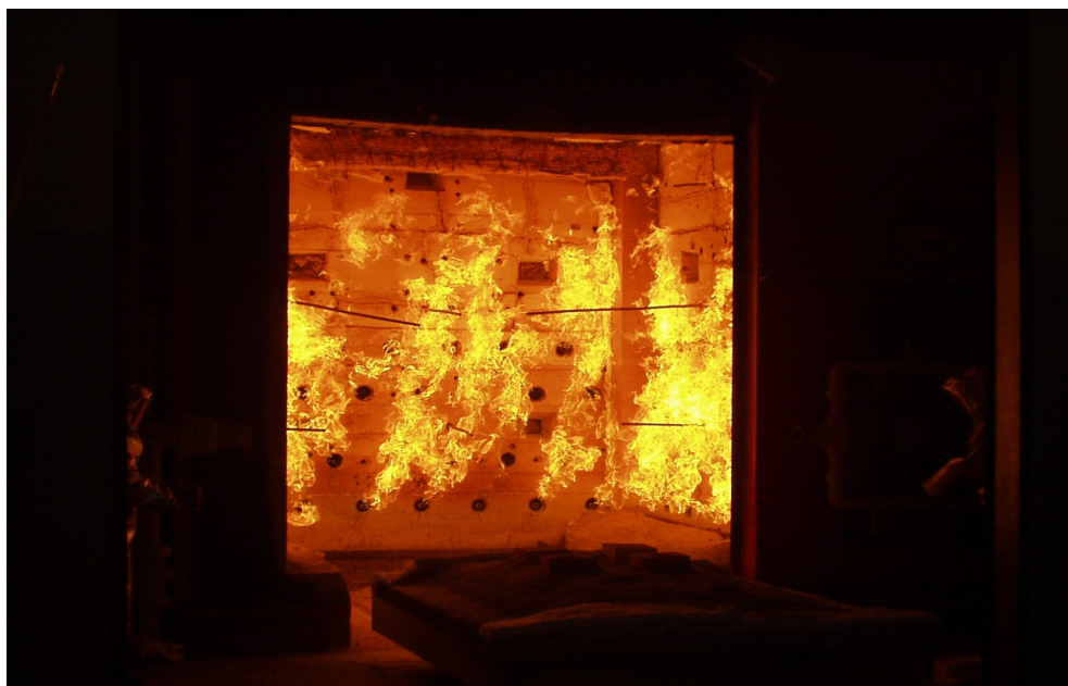
Figure 1—ASTM E119 Furnace Test of Fire Resistive Coating on a Structural Steel Column
